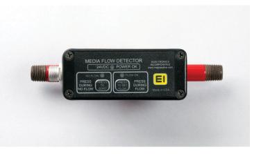
The MFD-250 Sensor uses a charge-coupled amplifier that is connected to a sensing pin placed in the flow path of the abrasive blasting media. Each particle passing the pin shares a minute charge with the pin, converting it to a voltage used to activate the output relay contact.
