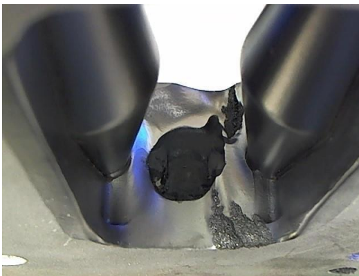
Figure 4: Severe erosion on pole pieces and casting resulting from prolonged media starvation.
