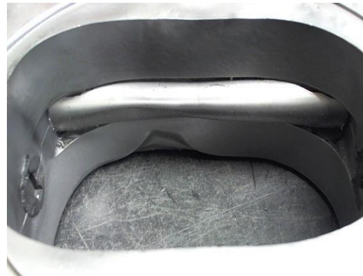
Figure 4: Severe erosion on pole pieces and casting resulting from prolonged media starvation.
